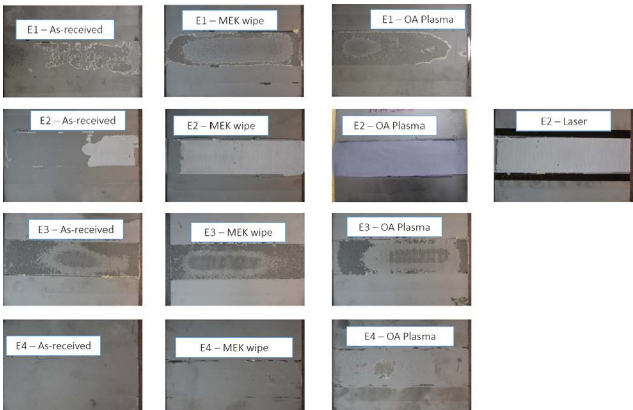
Figure 10. Images of peel tested specimens with epoxy adhesives E1, E2, E3 and E4, showing their failure modes
